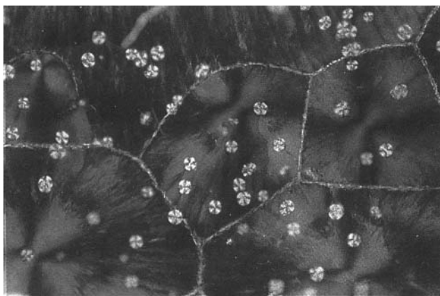
Figure 8 A semi-crystalline polymer electrolyte film of \text{PEO}_8\text{:LiClO}_4 photographed under crossed polarizers in a polarizing microscope.
